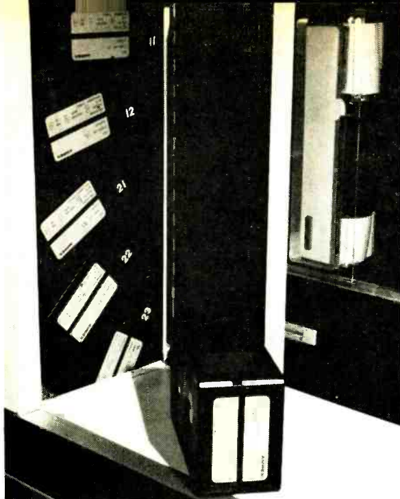
View of transport with carousel door open and five cassettes installed.
